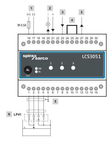
Item Power supply 2 Signal output 1 for external alarm 24 Vdc, 100mA (semiconductor output) 3 Safety circuit, input and output Wire link, fitted on site, when used as high water level alarm acc. to EN 12952/EN 12953 4 CEP Central earthing point in control cabinet 5 6 Level probe LP41
